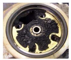
The photographs above are from an engine which has completed approximately 110,000 miles. The engine has been serviced by an approved dealer at the correct service intervals using the manufacturer's recommended oil and filters. This engine has caused two new turbocharger failures in a very short time.
