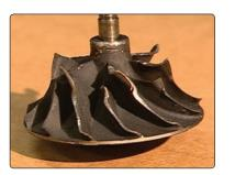
Even a very small foreign object can cause considerable damage to turbine or compressor blades. Foreign objects can enter the turbo due to careless maintenance, leaks in the air intake system or fragments from a failed turbo which have not been flushed through.
