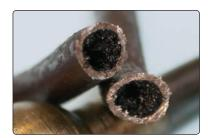
As a turbo operates at up to 6,000 revs per second, up to 950°C and to very fine tolerances, lubrication is critical. Running a turbo without oil for five seconds is as harmful as running an engine without oil for five minutes.
