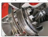
bertormance at all engine speeds. characteristics to improve engine Variable turbine turbos adapt turbo
