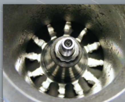
Any object sucked into the compressor will damage it
