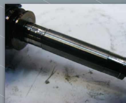
Extreme wear on the turbine shaft caused by oil contamination
