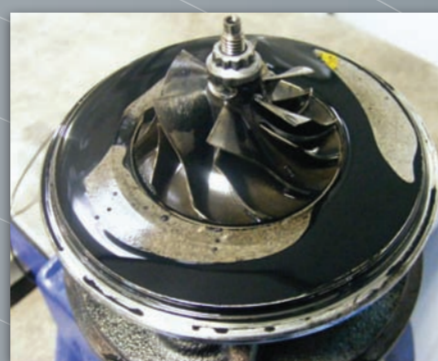
Compressor end oil leakage due to low air pressure
