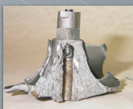
Compressor destroyed by overspeeding
