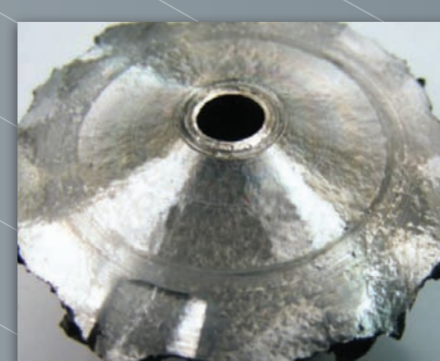
Orange peel effect on backface caused by overspeeding
