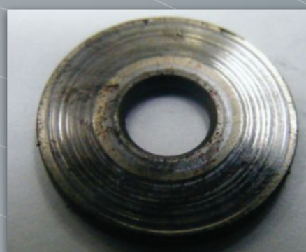
This marking is evidence of contaminated oil
